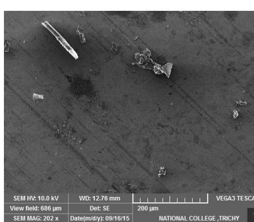
Fig. 50 Worn-out surface of gray cast iron
