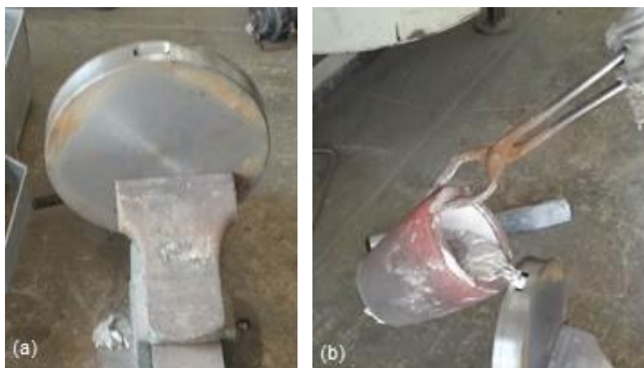
Fig. 10 Composites are casted in a cylindrical steel die, (a) before casting, (b) after casting
