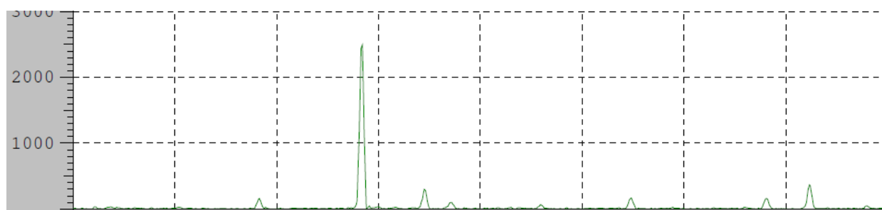
Fig. 17 XRD spectrum of A356 composite reinforced with 4% vol MWCNT
