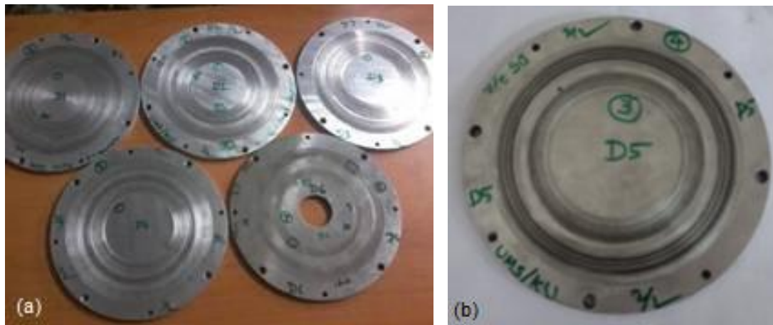
Fig. 28 Photographic view of the sample after wear test: (a) D1, D2, D3, D4 and D6 (b) D5
