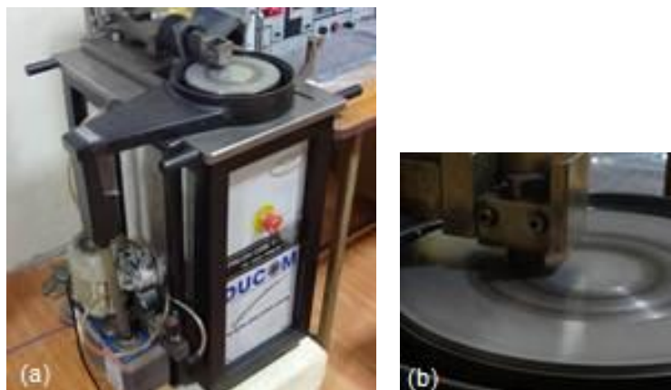
Fig. 27 DUCOM pin on disc apparatus: (a) experimental set-up, (b) contact between pin and disc
