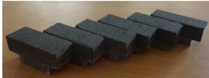
Fig. 26 Pins prepared from Car Brake pad Material
